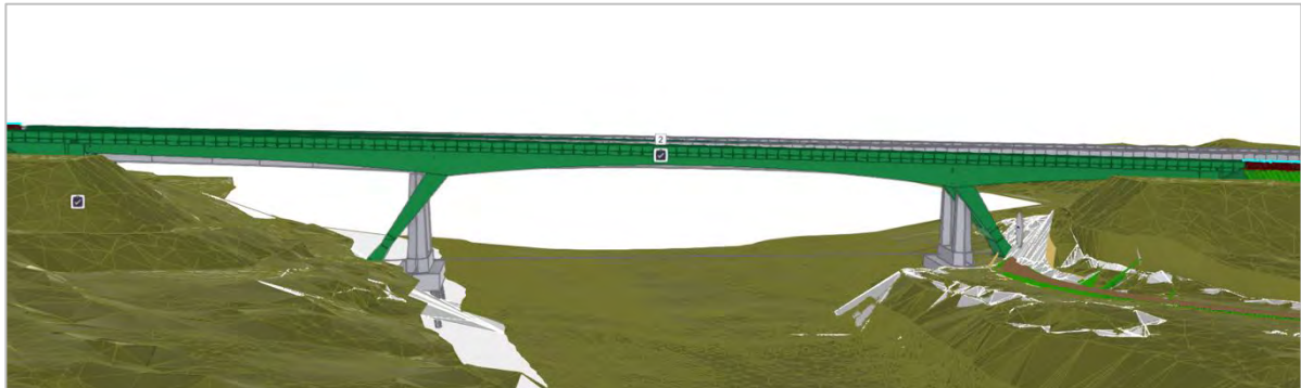
Figure 3: Before (grey) and after (green) images from the project BIM of the new Turku Bridge design that resulted in a €12m saving. (source: aki.kopra@kreate.fi 2 )
